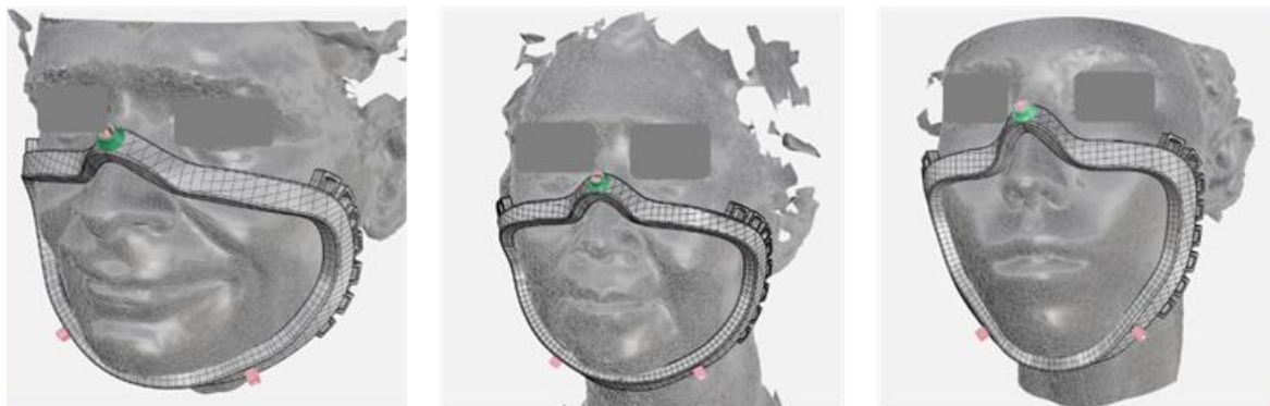
Figure 13. Digital prototypes of custom-fit RPD Frames on three subjects.
