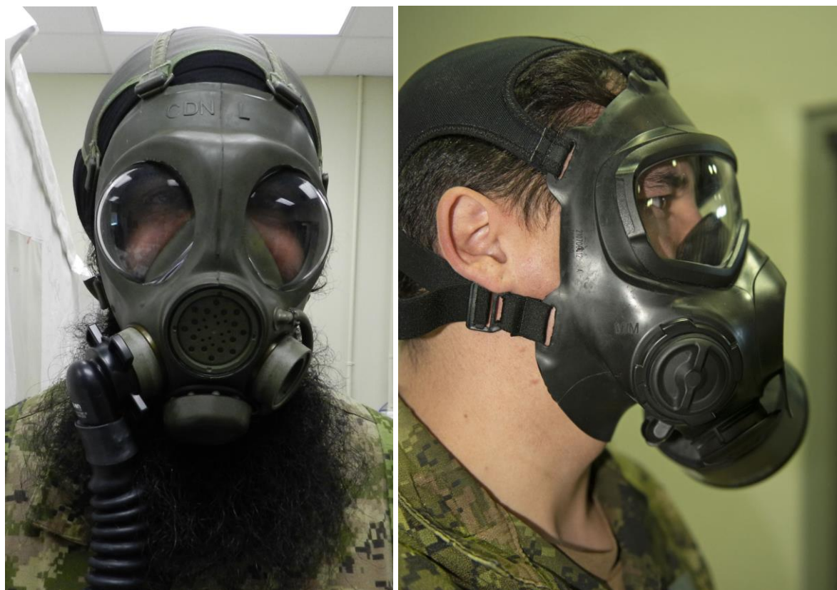
Figure 1. Left: C4 respirator in PAPR mode worn by individual with beard and headdress; right: C5 respirator with C8 canister worn by individual without a beard or headdress in normal, non-powered mode.
