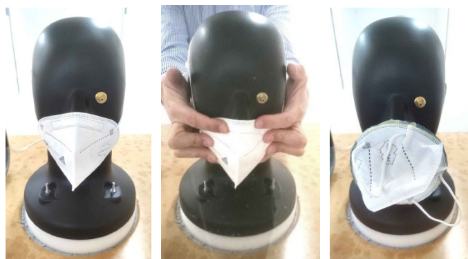
Figure 5: Test configurations of one negative-pressure P2 filtering facepiece respirator with ear loops (PPETECH).
