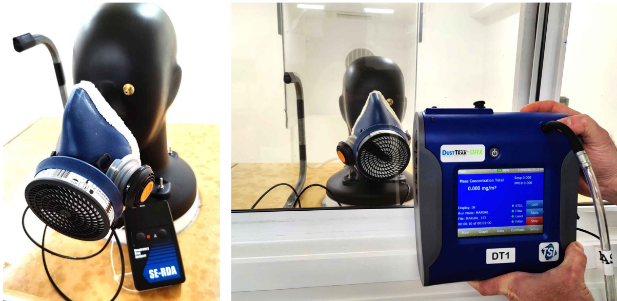
Figure 15: Pressure and flow are logged by SE-RDA logger during the test. Concentration inside the chamber is 34.1 \text{ mg/m}^3 , inside the respirator is 0.000 \text{ mg/m}^3 .
