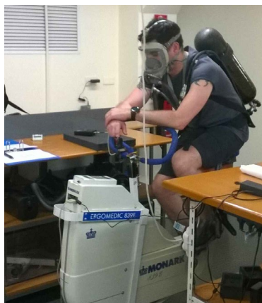
Figure 18: Monark bicycle ErgoMedic 839E (with SCBA + Full-face mask. Tested for reference).
