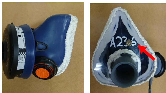
Figure 8: Modified Sundström mask SR100 and Filter SR510 with orifice fitted.
