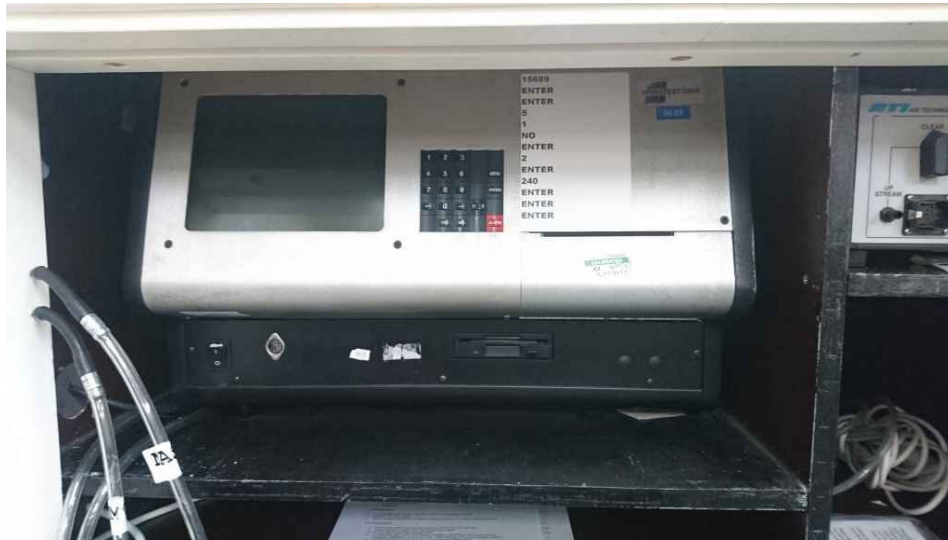
Figure 2: Breathing machine to simulate human breathing.
