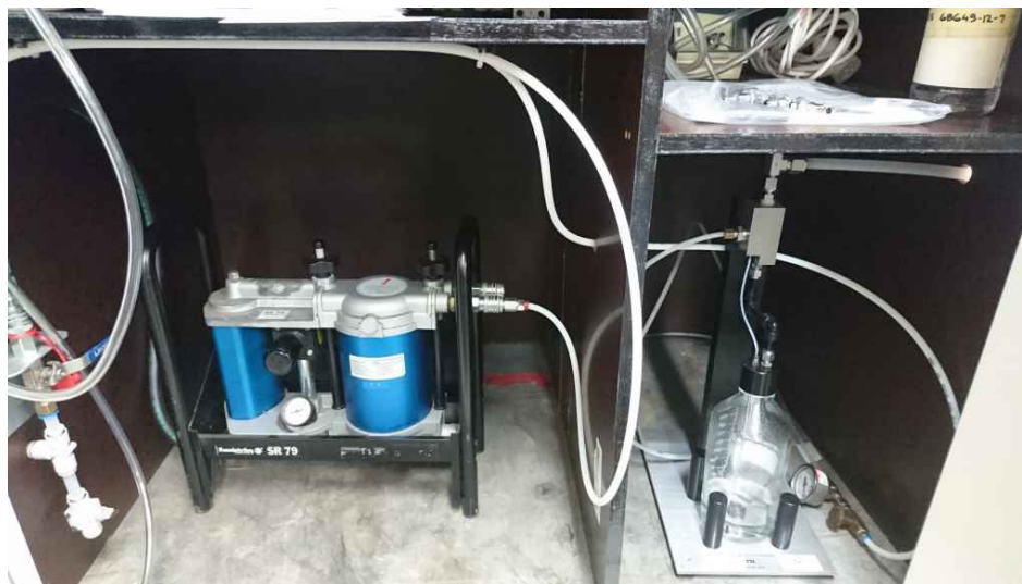
Figure 4: Pressure/flow source and atomizer to generate the particles.
