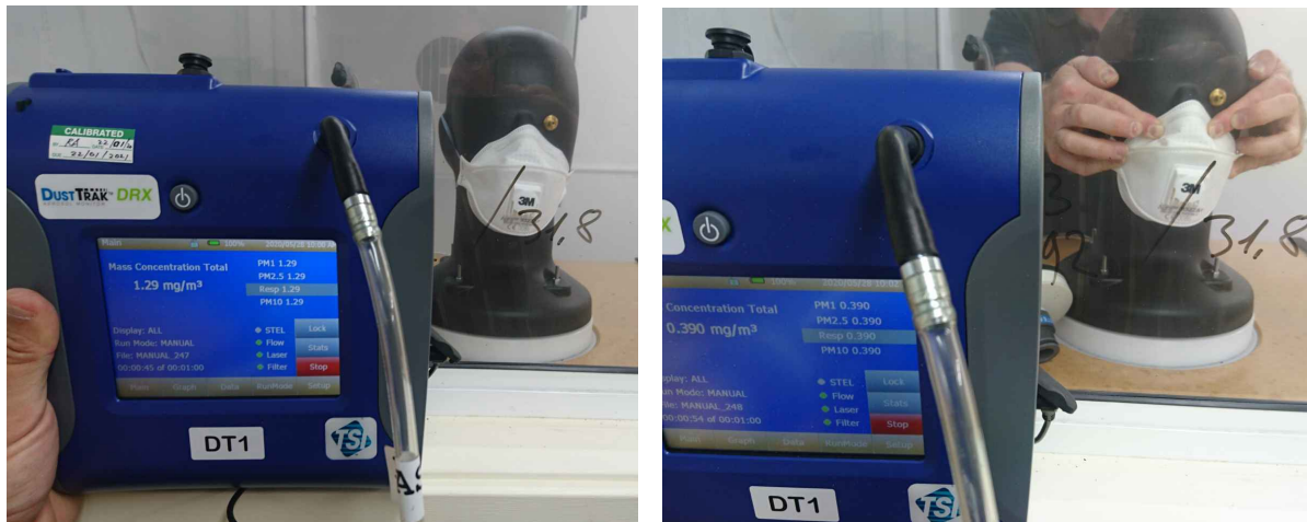
Figure 6: 3M filtering facepiece respirator mounted on the headform (left) and edges of the respirator forced to the face to improve the face seal (right).
