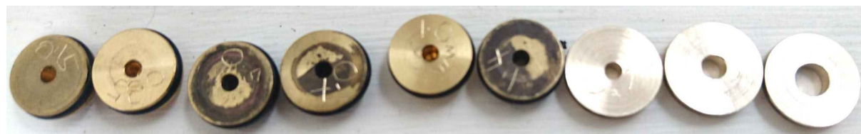
Figure 9: A set of calibrated orifices was used to simulate controlled breakage of face seal (0.15-4 mm).
