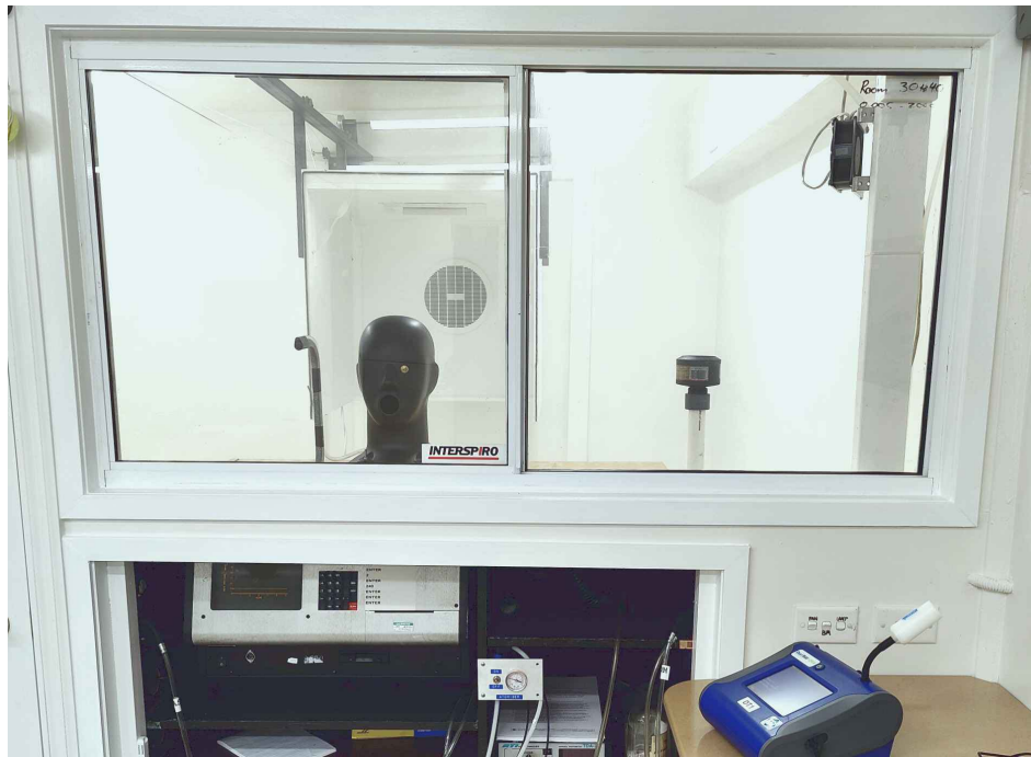
Figure 1: SEA Test chamber with the test head connected to the Breathing machine (below).
