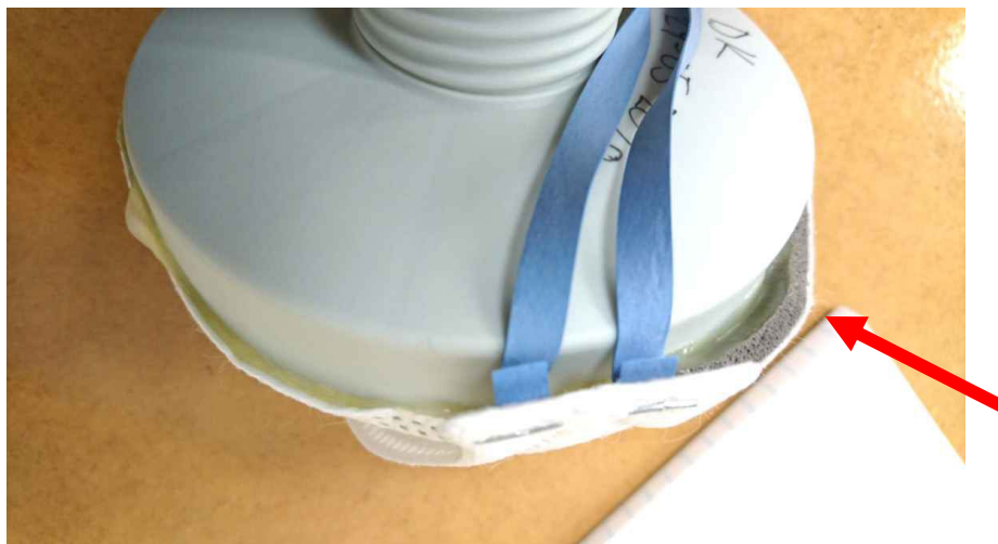
Figure 7: 3M respirator is glued to the test plate. The arrow points to the foam on the nose bridge.
