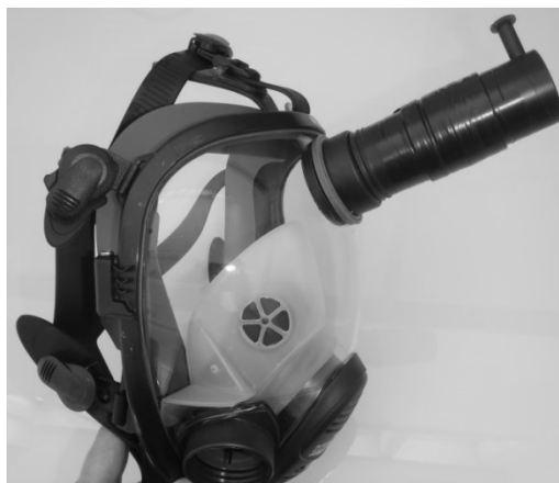
Figure 2: Modified mask to allow sampling of asbestos fibres.
