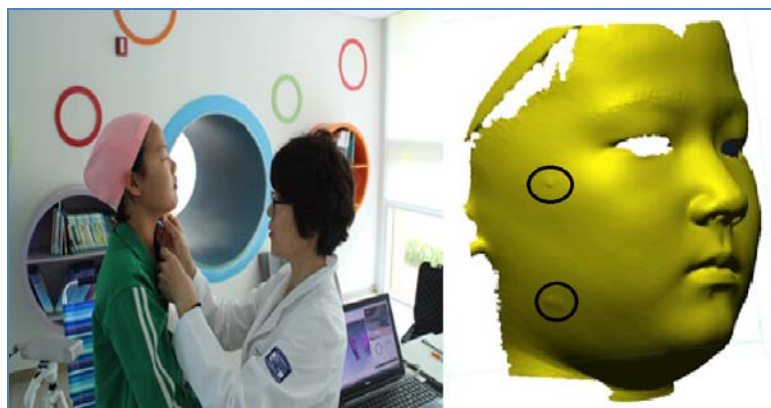
Figure 2. Placing landmarks on the subject's face (left) and the land marks appeared after scanning (right).
