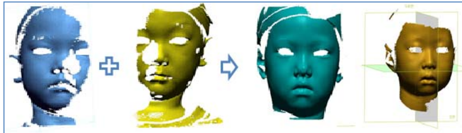
Figure 3. 3D Modeling processes showing merging and registration of scanned data.
