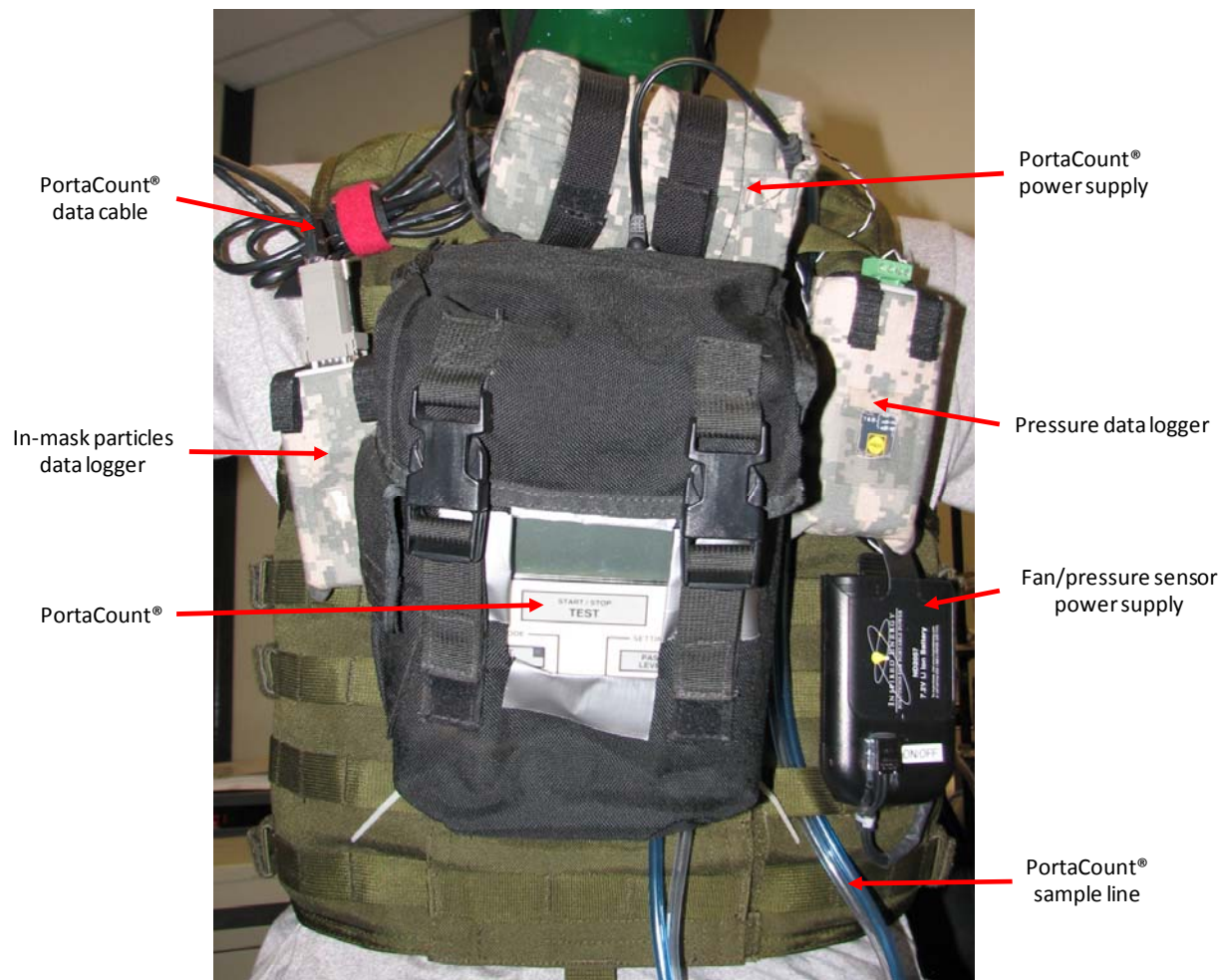
Figure 2. Load-bearing vest instrumented with data acquisition components.
