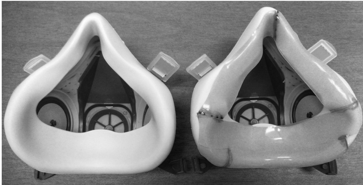
Figure 2. A conventional and modified elastomeric half-mask respirators (same model).
