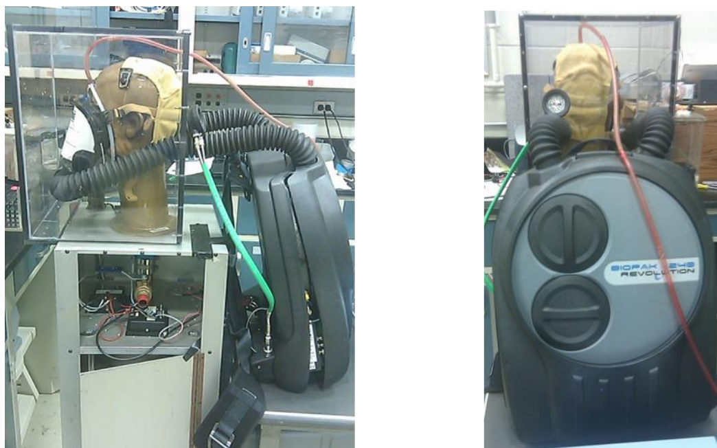
Figure 4. Overall test setup with the SCBA facepiece mounted on the breathing machine head form.
