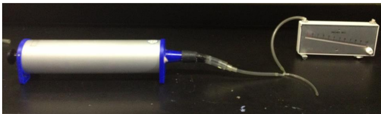
Figure 2 Leak assessment setup. A hand operated syringe was pulled to match the pressure found in the facepiece of a CC-SCBA to determine the leak rate from various tube sizes which were inserted into the facepiece.
