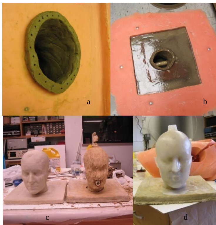
Figure 2. Headform fabrication: (a) Mold lined with clay to create void space, (b) Clay lined mold filled with expanding foam to form supporting core and base, (c) Expanding foam cast (left) and expanding foam core with clay removed, (d) Expanding foam core overcast with skin-analog silicone.
