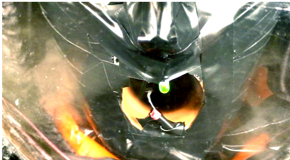
Figure 1. One frame of a video taken during a fog challenge test. This picture shows fog inside the face area of the Centurion MAX. The picture is of the black head form mouth area with green LED in the region of the upper lip and fluttering string at the base of the bottom lip.
