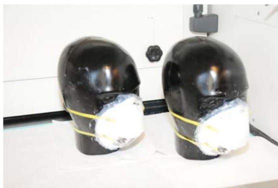
Figure 1. Sealed N95 FFR on the manikin head.
