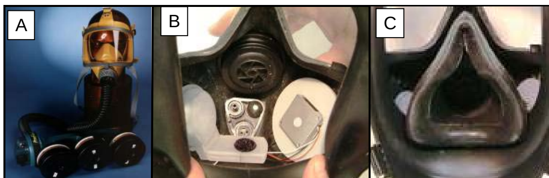
Figure 2. A) Commercially available PAPR device. B&C) Internal modifications made to the standard negative pressure respirator to create the dual cavity prototype. The miniature blower unit can be seen in the lower right hand side of the B.
