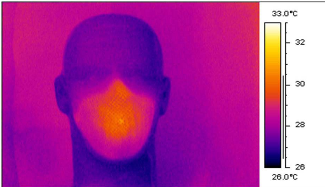
Figure 1. Infrared camera image of N95 filtering facepiece respirator during end exhalation.
