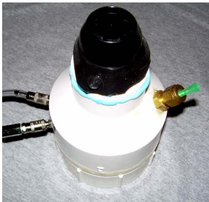
Figure 1. Sealed canister fitted with exhalation valve and hypodermic needle.
