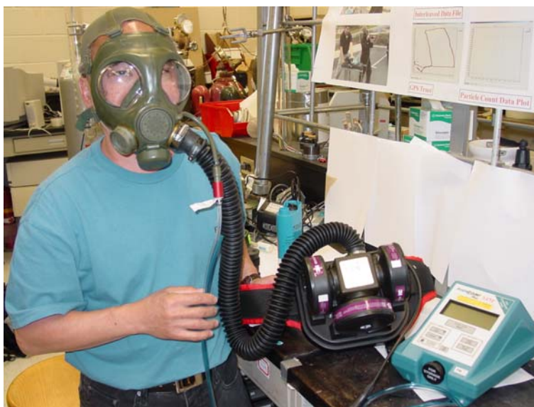
Figure 1A. The 3M BE-10 blower system connected to a PC4 mask.
