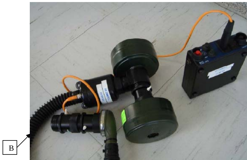
Figure 1B. The Carlton blower [Note: B indicated the adapter where this system normally screwed onto the C4 mask at the canister mount].
