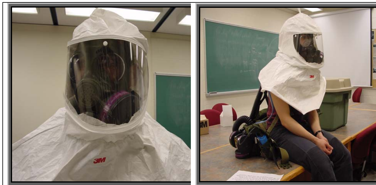
Figure 2. 3M Breathe Easy hood surrounding the gas mask (left) and 3M hood and the blower system (right).
