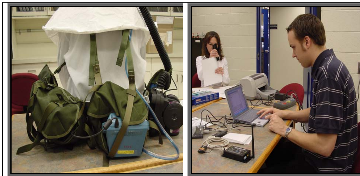
Figure 1. Portacount and blower mounted on CF webbing (left) and base station to record data from the Portacount (right).
