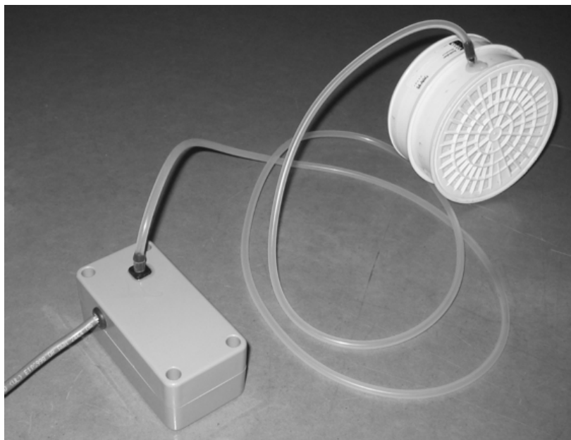
Figure 3. Flow meter assembly, comprising filter, flexible tube, and pressure transducer.
