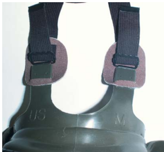
Figure 2. Placement of padding beneath the buckles of the M40 forehead straps for the Padded M40 condition.
