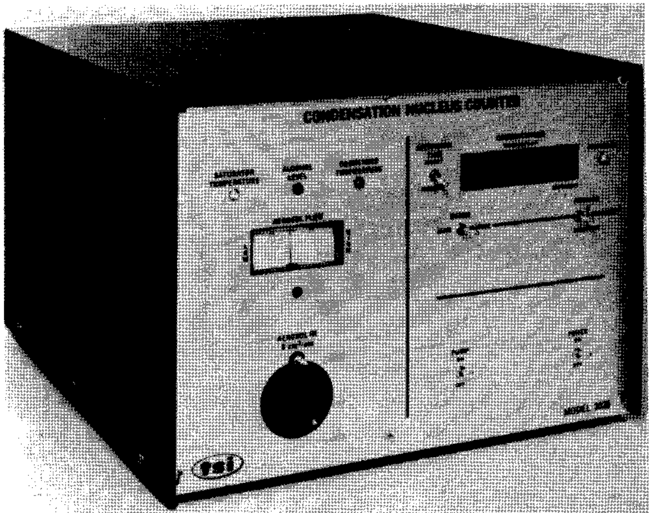
Figure 2. TSI Model 3020 condensation nucleus counter.
